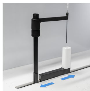
Figure 3. RidingRinse integrated to 4DXW autosampler.
